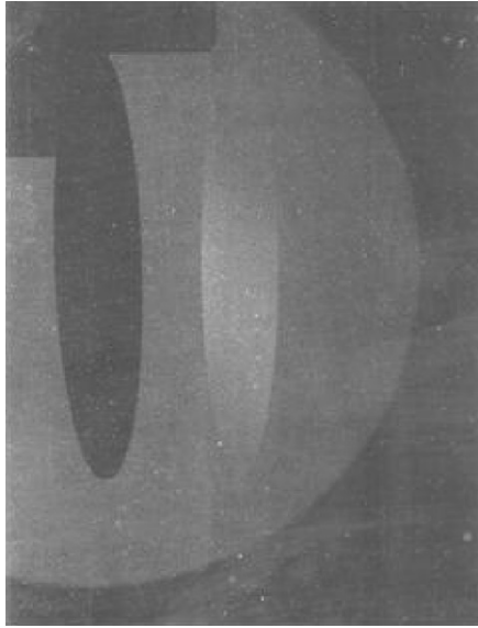
Fig. 7. Radiograph using the PXR beam that reflects by the arrangement “+ - +” with a Polaroid film.
