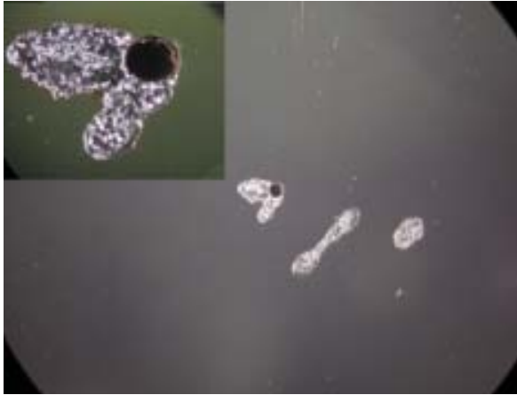
Figure 4: Damages on the surface of the Ag coated silicon. Entire mirror (25mm in diameter) and close up around the coupling hole.
