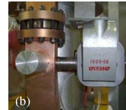
Figure 5: The Photograph of the PV-3040N klystron. (a) Overview of the PV-3040N klystron. (b) Close-up around the klystron ion pump.
