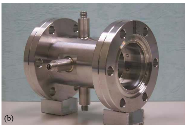
Figure 2: Geometrical drawing (a) and photograph (b) of the Stripline-type Beam Position Monitor.
