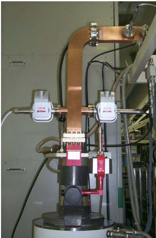
Figure 3. The photograph of the waveguide with two additional vacuum pumps downstream the klystron RF window
