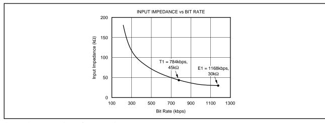
CURVE 3. Input Impedance of rxLINE and rxHYB.
