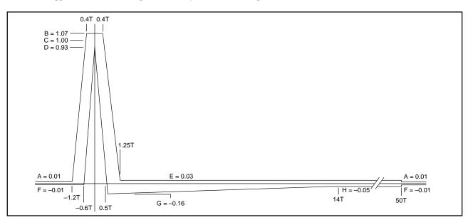
CURVE 2. Transmitted Pulse Template and Actual Performance as Measured at Transformer Output.
