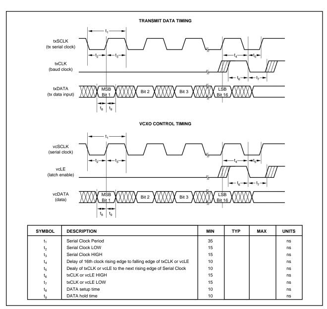
FIGURE 4. Timing Diagram.
