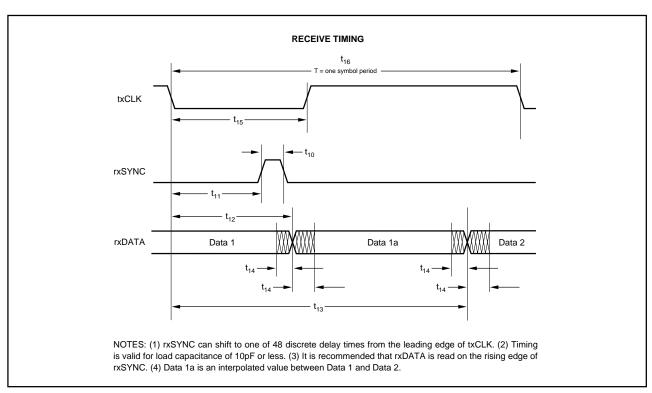
FIGURE 5. Receive Timing Diagram.
