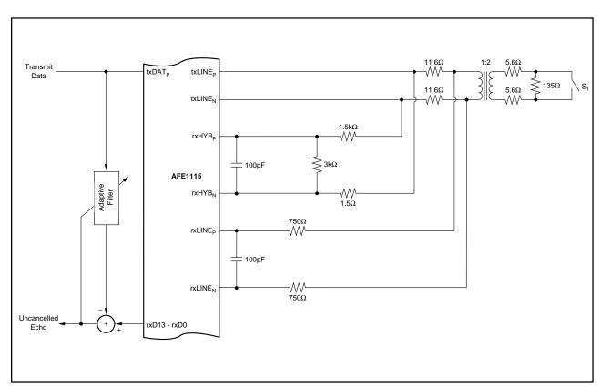
FIGURE 6. Uncancelled Echo Test Diagram.
