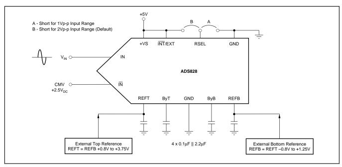
FIGURE 8. Configuration Example for External Reference Operation.
