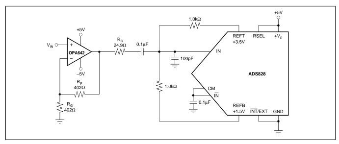
FIGURE 3. AC-Coupling the Dual Supply Amplifier OPA642 to the ADS828 for a 2Vp-p Full-Scale Input Range.
