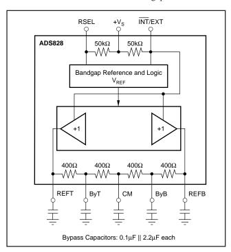
FIGURE 6. Equivalent Reference Circuit with Recommended Reference Bypassing.
