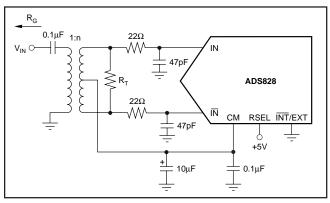
FIGURE 5. Transformer Coupled Input.
