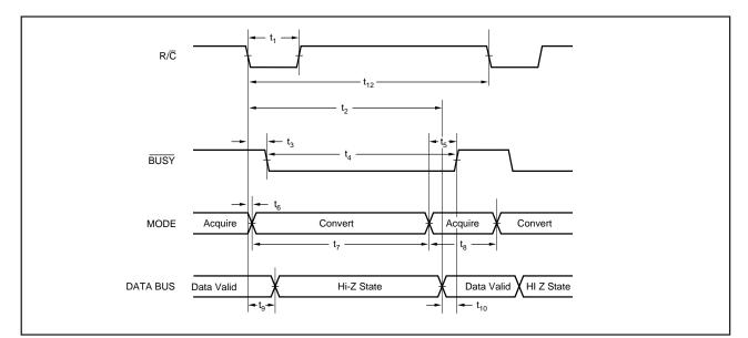
FIGURE 2. Conversion Timing with Outputs Enabled After Conversion (CS Tied Low).
