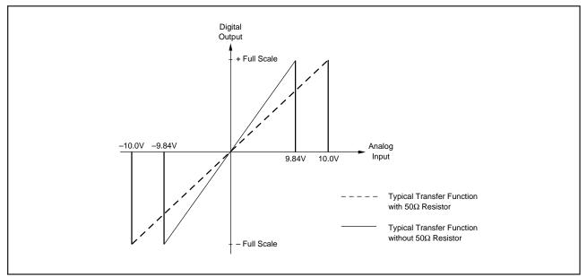
FIGURE 5. Comparison of the ADS7810 Transfer Function With and Without the 50Ω Series Resistor on V<sub>IN</sub>.
